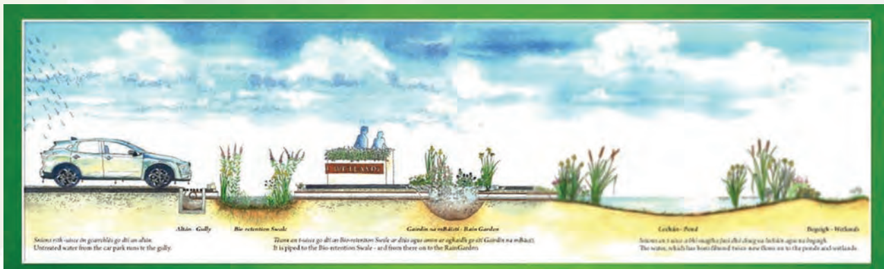
Figure 15: Diagram showing urban SuDS in action.
