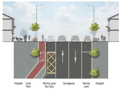
Proposed: a reduction in the total width of the carriageway could allow for a cycle lane and spill out areas for cafés, with seating and improved street furniture.
