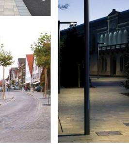
TL: Use of differentiated paving to strengthen the visibility of the crossing TM: Cycle physically separated from traffic on the main street
