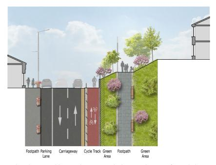
Proposed: redesign Dublin Road section with the introduction of a cycle lane and of a footpath protected from adjacent traffic.
