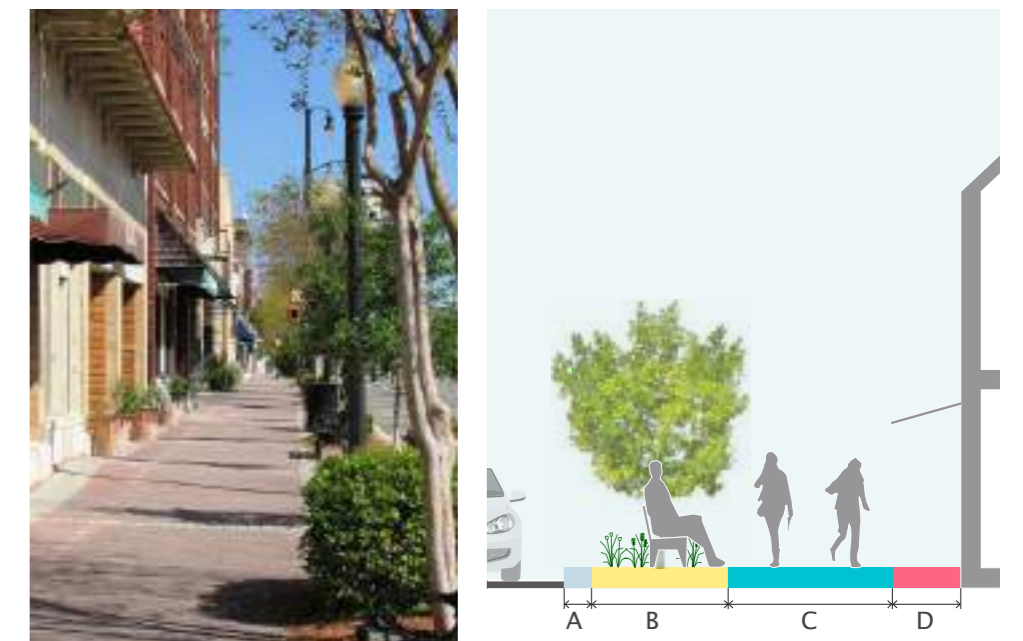
L: Pavement of the main street of a small town, with a landscaped buffer zone R: Location and width of footpath zones as described above.
