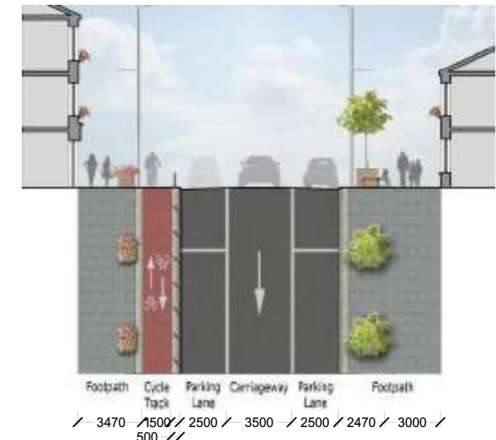
Proposed: potential redesign of Main street will allow for a single lane of traffic, and the public realm space could be maximised by removing perpendicular parking bays. A dedicated cycle track could be introduced, together with a planting and seating zone.
